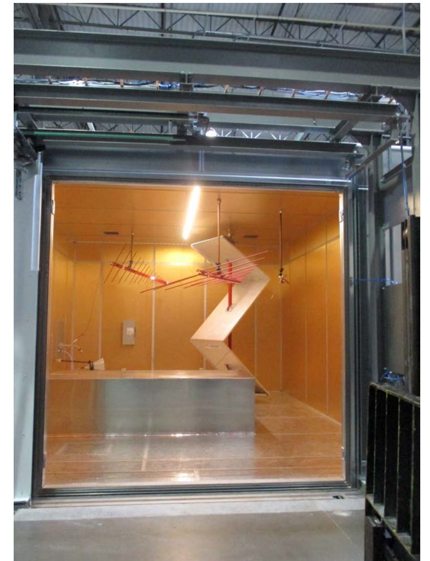
Reverberation chamber at NTS Plano.
