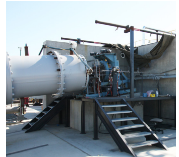
Front and side view of the Thrust Measuring System
