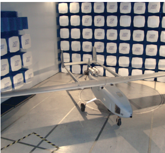
UAV testing in an EMI chamber at NTS Plano, TX
