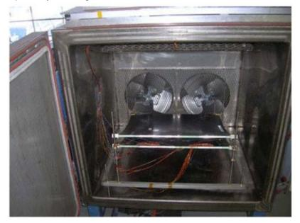
Coupons in a Positive-Pressure Nitrogen Test Chamber
