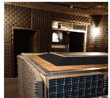
Combined vibration, temperature and sound test chamber
