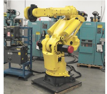
Robotic operation integrated with environmental chambers for continuous ambient/hot/cold/humidity cycling.
