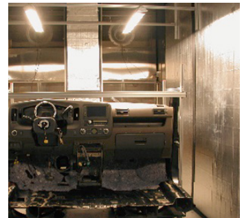
Solar radiation exposure testing of automotive dashboard
