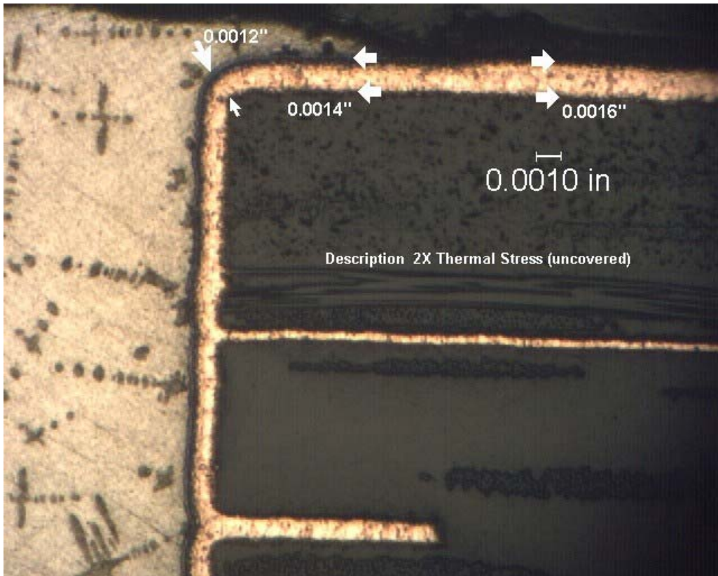
Photo 5: Vendor A, 2X Thermal Stress, Uncovered
