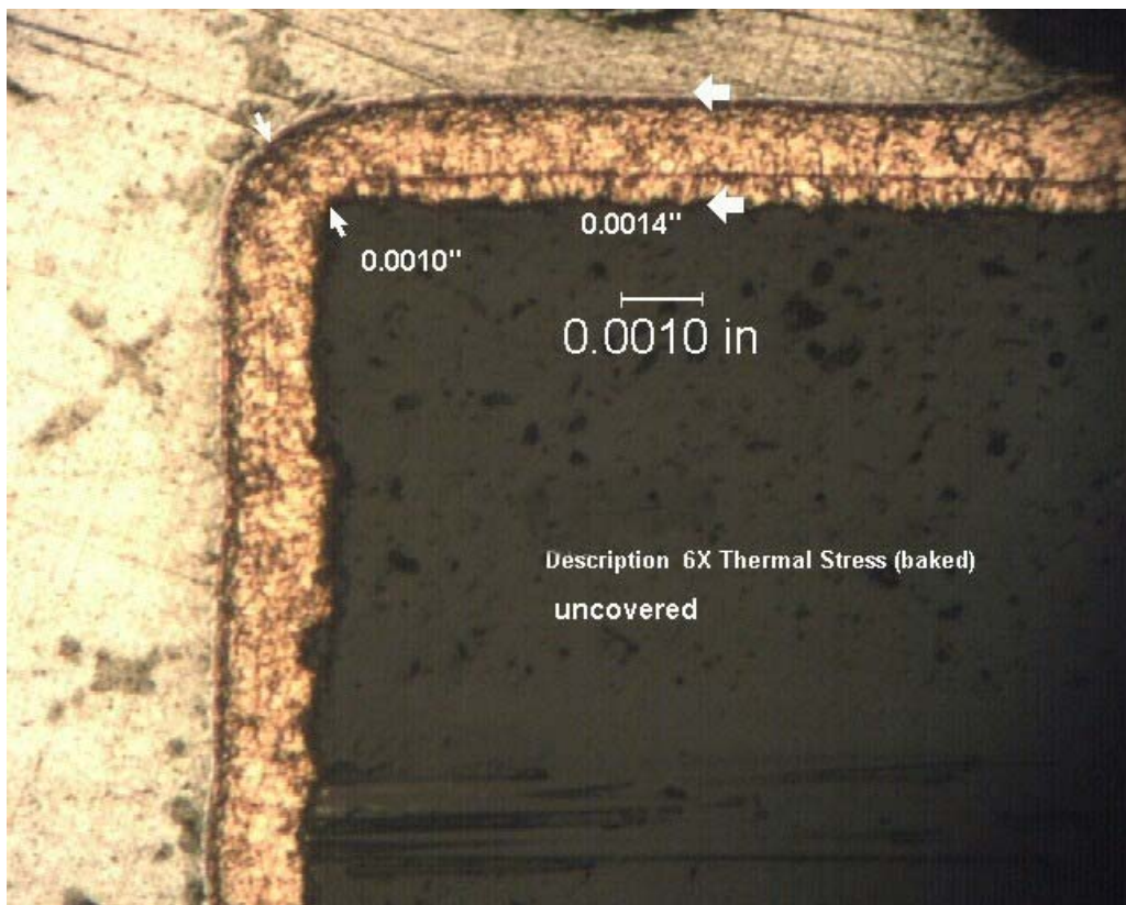
Photo 13: Vendor A, 6X Thermal Stress, Uncovered
