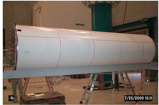
Figure 8 Typical Arrangement of Conductors on 1/60 Scale Model Test Article
