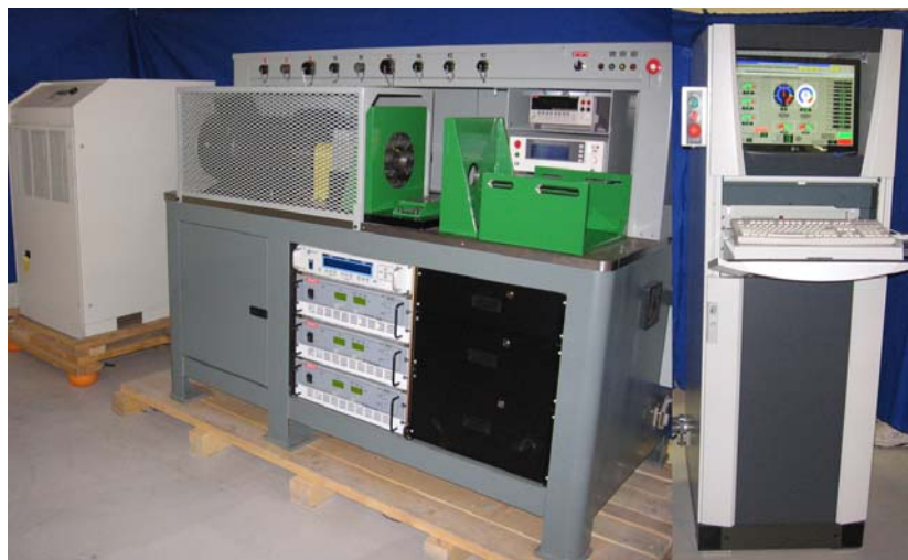
Figure 1, Multiple Electric Motor Test Stand
