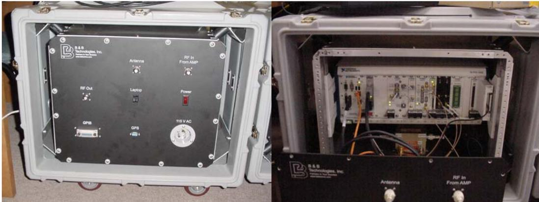
The PXI chassis packaged with other RF components in a shippable container.
