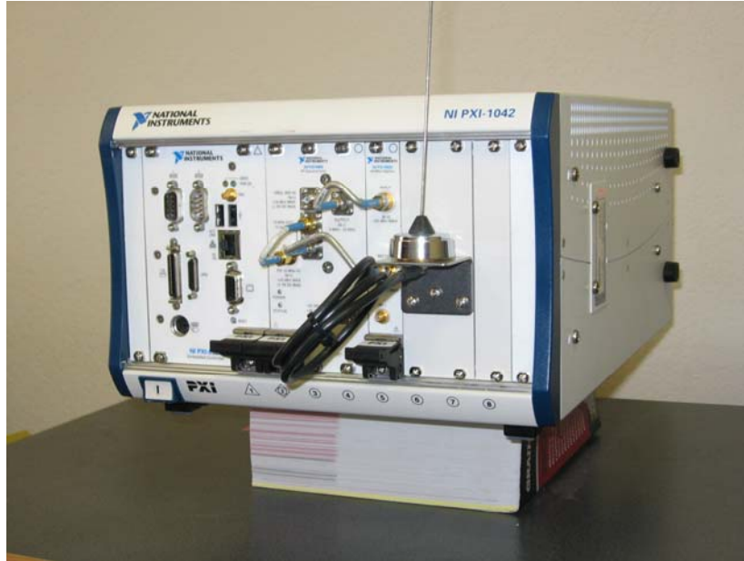
Figure 1. RF Components Tester for Wireless Security Systems
